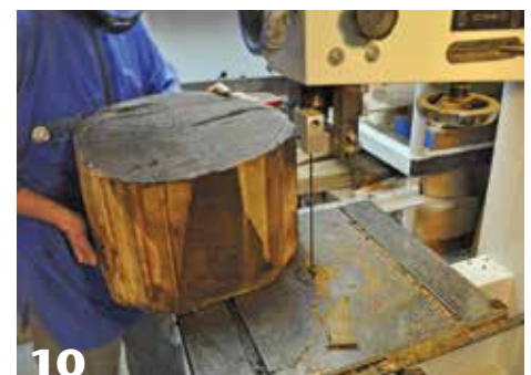
A bowl blank can be rough-shaped with a chainsaw, or by using a bandsaw. Both bowl blanks will become large, deep, one-piece bowls, which could not be accomplished using kiln-dried stock.
