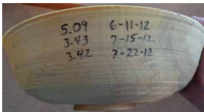
A 13"- (33cm) cottonwood bowl, rough turned from green wood, weighed 5.09 lb (2.3kg) June 11 when it was placed in the kiln. It weighed 3.43 lb (1.6kg) July 15, and 3.42 lb (1.6kg) July 22. This bowl stopped losing weight, is dry, and ready to be finish turned.
