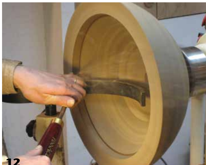
12 After air-drying this walnut bowl blank for several months, it can be finish-turned.
