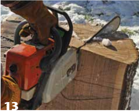
Spindle stock can be cut using a chainsaw, or, alternatively, a bandsaw.
