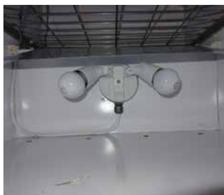
The lightbulbs are mounted on the back of the kiln near the bottom, a sheet of metal covers the bulb, and the holes are drilled through the bottom of the freezer.
