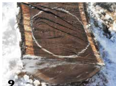
A bowl blank can be rough-shaped with a chainsaw, or by using a bandsaw. Both bowl blanks will become large, deep, one-piece bowls, which could not be accomplished using kiln-dried stock.
