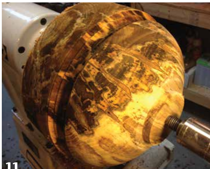
11 Rough turning the outside of a maple bowl from green wood reveals mineral streaks and ambrosia markings.
