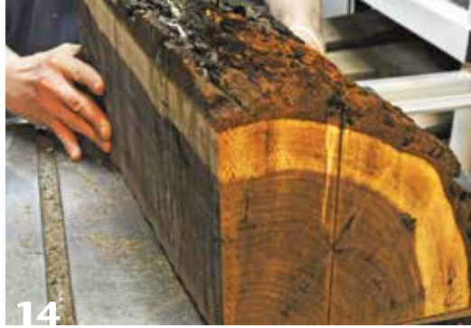
Spindle stock can be cut using a chainsaw, or, alternatively, a bandsaw.
