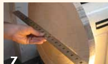
7 Use a straight edge across the entire diameter to test for flatness, not only at the rim area, but also across the entire board. It may be helpful to shine a light from under the straight edge to highlight any gaps.
