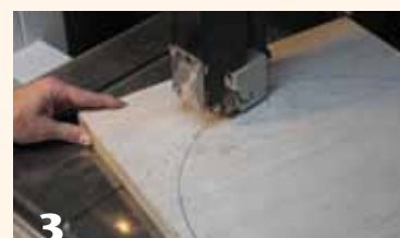
3 Measure, mark, and then cut the rim material to approximate diameter. Mount the rim material onto the lathe.
