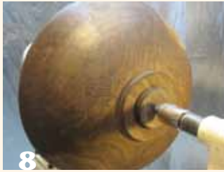
8 Mount the rough-turned bowl onto the lathe. A jam chuck along with the tailstock for support works well. Turn the tenon and outer walls back into round.
