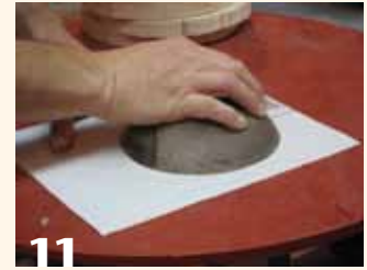
11 Minor adjustments to the bowl's rim and to the rim material can be made by hand sanding against a surface you know is flat.
