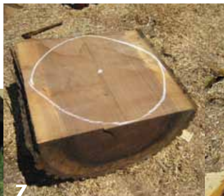
7 This half log will make an attractive walnut bowl. The circle encompasses almost equal amounts of sapwood on either side. Drawing a circle with a piece of chalk is a helpful aid when using a chainsaw to rough-cut a circle.
