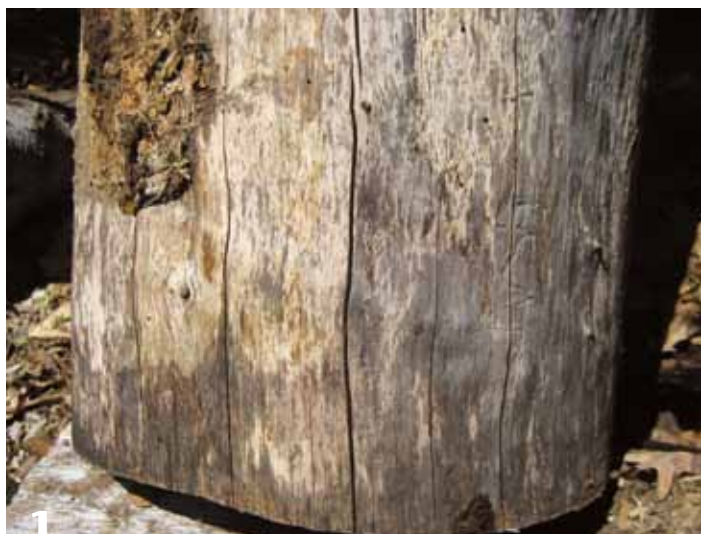
1 Surface checking on a maple log. The deeper the cracks, the less usable wood there is to harvest from a log.
