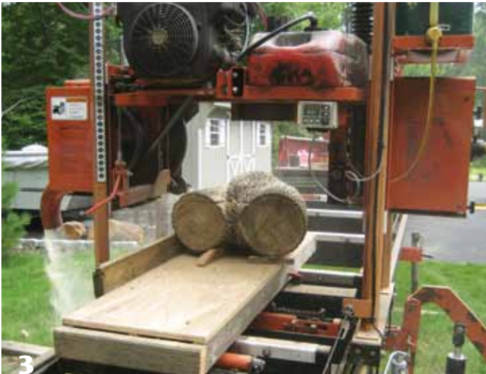
3 A horizontal cut through this ash crotch required a bit of wedging to stabilize the log. The sawmill delivered precise placement of cuts, which resulted in wood that was easier to process and also minimized waste.
