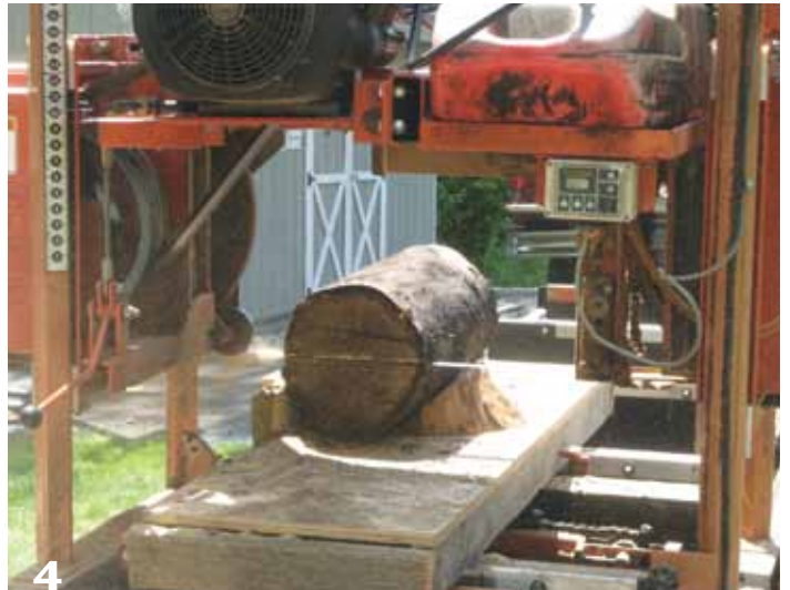
4 Our sawmill setup consisted of a wooden platform with a fence and wedges to hold the logs in place.
