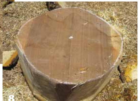
8 Now that the half log is cut into a rough circle, it will be safely mounted onto the lathe for roughing into a bowl blank, then cored.
