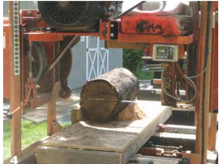
4 Our sawmill setup consisted of a wooden platform with a fence and wedges to hold the logs in place.
