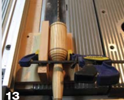
13 Clamp the taper to the jig. Raise the table saw blade only high enough to cut through the jig and only one side of the taper. The cut should stop a bit short of the bottom of the tone chamber.
