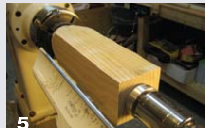
5 Here the piece is mounted, drilled out, and supported with the cone center.
