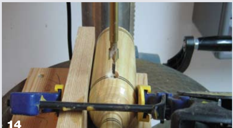
14 Drill a \frac{3}{8} " (10mm) hole at the end of each cut line.
