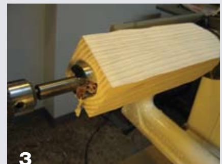
3 Using a 1½" (40mm) Forstner bit chucked in the tailstock, drill a hole 3"–4" (80mm–100mm) deep.
