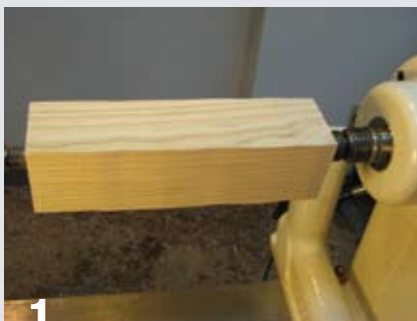
1 Mount the block between centers.
