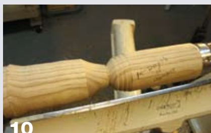
10 Begin shaping the handle at the left-most pencil line.
