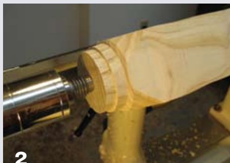
2 Form a tenon at the tailstock end.
