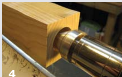
4 Use a cone center inserted in the tailstock for additional turning support.
