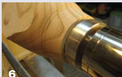
6 Begin at the tailstock end and turn the walls to about \frac{1}{8} " (3mm) thick.
