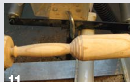
11 Form the handle and sand the taper.
