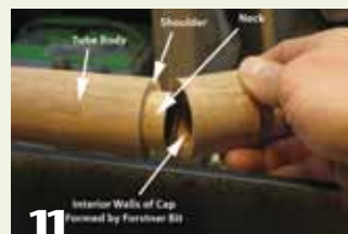
11 At this point, the cap should fit snugly and the outside of the tube is ready for final forming.
