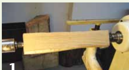
1 It is important to use dry wood, otherwise the piece could change shape after completion, altering the fit of the cap.
