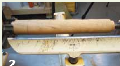
2 Turn the wood to a cylinder with tenons on each end. Mark the length for the cap.
