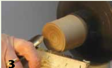
3 To cut across endgrain, engage the cylinder's edge slowly and carefully, then ride the bevel all the way to the center.
