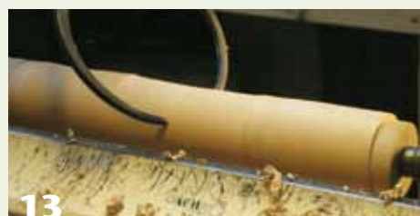
13 Measure the correct diameter at one point on the tube's body.
