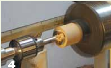
4 A Forstner bit quickly and consistently forms the interior walls of the cap.
