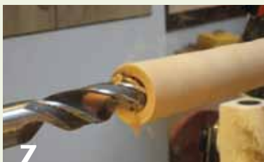
7 Drill out the tube's body slowly, clearing the chips frequently.
