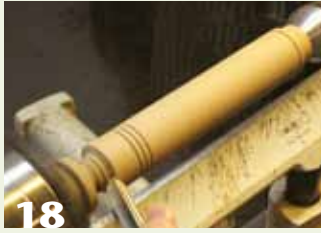
18 Use a spindle gouge to shape the bottom of the tube to create a decorative and smooth surface.
