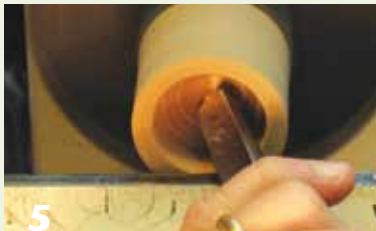
5 Cut from the center to the outside, with the bevel rubbing.
