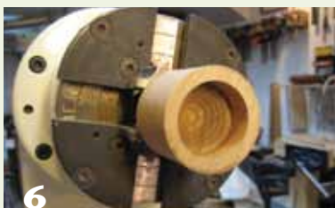
6 The inside of the cap is finished.
