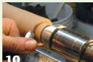
10 Cut the shoulder slightly concave. The principles used to create a good fitting cap are the same as those in making a lidded box.
