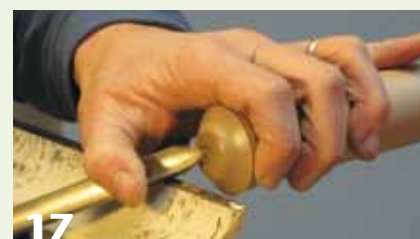
17 With the tailstock out of the way, apply counterpressure with your fingers for support when shaping the top of the cap.
