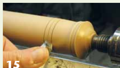
15 Turn V-grooves using a skew chisel. Here is where you can be creative with this project—there are many options for embellishment.
