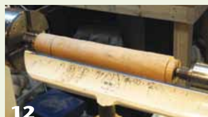
12 With a good friction fit, the cap and body are mounted together, ready for shaping the outside to achieve a seamless look.
