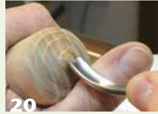
20 Remove the nub using a carving gouge, then sand.
