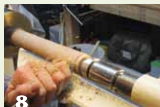
8 Use a cone center in the tailstock for support when beginning to form the neck section.
