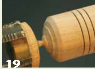
19 Leave a nub of wood attached to the bottom and use a handsaw to part the cylinder off.
