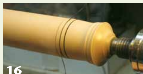
16 Using a wire, burn the V-grooves to highlight them.
