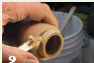
9 Use your fingers to apply counterpressure as you fine-tune the neck to achieve a perfectly fitting cap.
