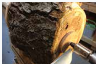
I formed a tenon to mount into a four-jaw chuck.
