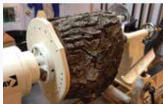
I screwed a plywood disc to the solid wood and screwed the disc to a faceplate.
