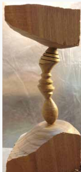
The ant bodies were my first attempt at multiaxis turning.
