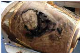
The initial forming of the vessel began to reveal its ant-hollowed interior.
