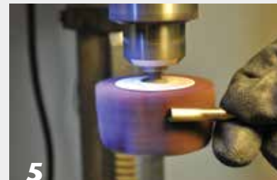
5 Lightly sand the brass tube before gluing it into the wood.
