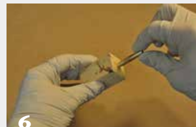
6 Lightly sand the brass tube before gluing it into the wood.
