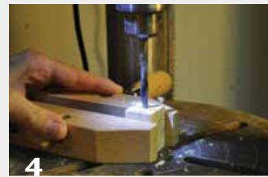
4 Drill a 7 mm hole through the wood. A wooden clamp will suffice to hold the piece, but specialized pen-drilling vises are available.
