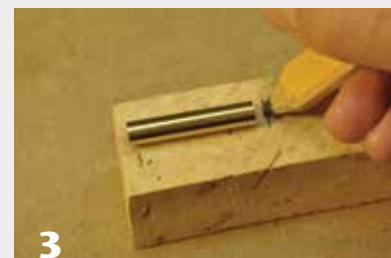
3 Cut the wood about ¼" longer than the brass tube, allowing for ⅛" of wood beyond each end of the tube.
