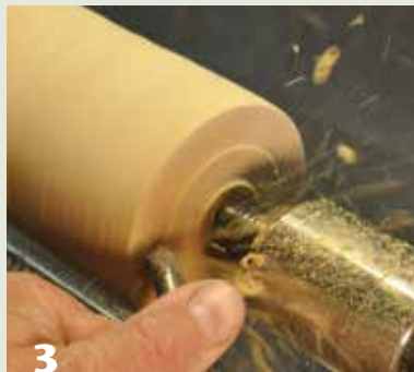
3 Cut across the endgrain to achieve a clean cut.
