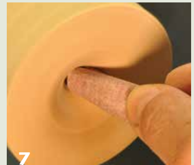
7 Sand the opening to soften the opening of the hole.
