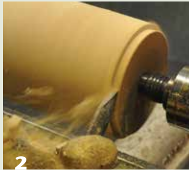
2 Form a tenon, sized to fit your chuck.
