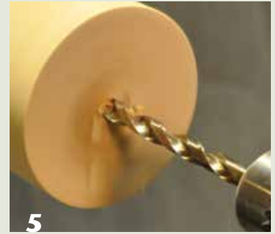
5 A Jacobs chuck in the tailstock is an easy and accurate way to drill on the lathe (see sidebar for safety note).
