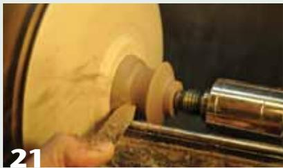
21 Shape the knob using either a round-nose scraper (l) or a small bowl gouge (r).
