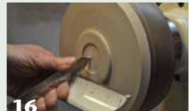
**16** With the lid jam fitted onto the body, cut a recess into the center of the lid to receive the tenon on the knob cylinder.
