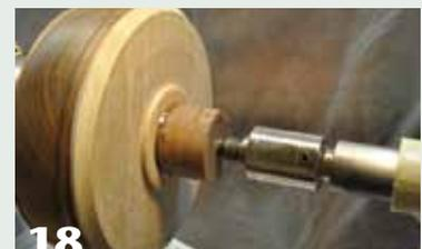
**18** Glue the knob into the recess and use the tailstock as a clamp.
