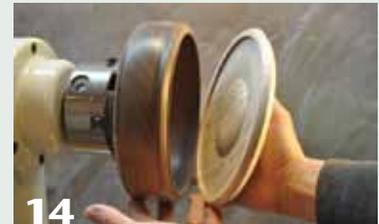
**14** The inside of the lid fits over the lip of the body and for the next step, a jam fit is required.
