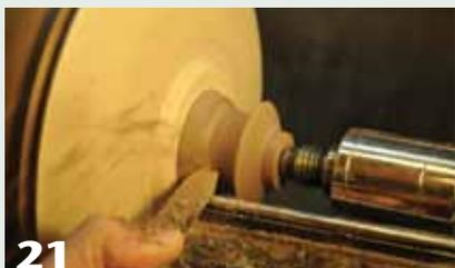
Shape the knob using either a round-nose scraper (l) or a small bowl gouge (r).
